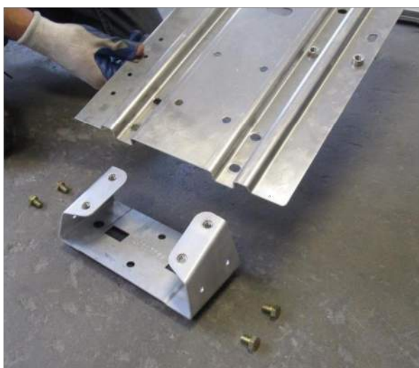
STEP A – INSTALL REAR LEG TO RAIL
