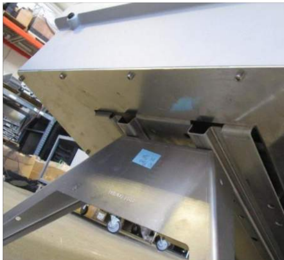
STEP B – ALIGN MOUNTING TAB WITH INVERTER SLOT
